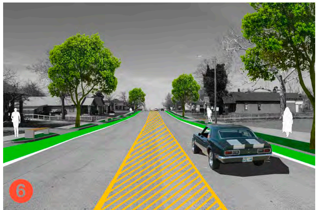
View of striped median buffer, bike lanes, and new street trees in residential area.
