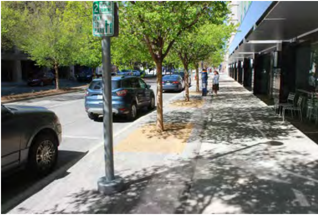
Street trees, lighting, and furnishing can be located in an amenity zone adjacent to the sidewalk. Project 180, Oklahoma City.
