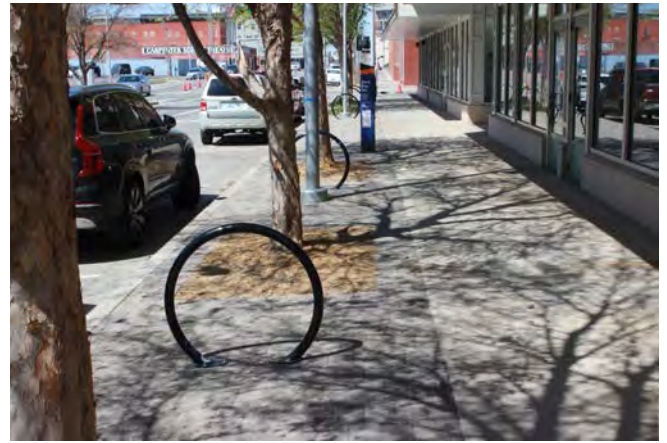
Bicycle parking can be located in the pedestrian amenity zone. Project 180, Oklahoma City.
