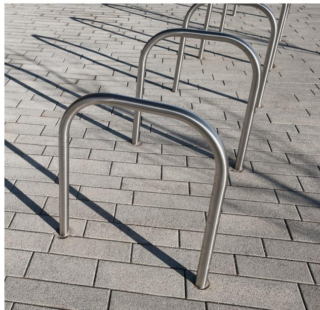
Inverted U-shaped racks are the most common, allowing for enough space for bikers to come and go. These bicycle racks are typically bolted to the ground and are sturdy enough to hold the bike without the bike falling over. They allow for two points of ground contact and come in many variations.
